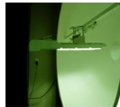
An integrating sphere is used to characterize lamps in order to obtain the total luminous flux, chromaticity coordinates (x, y), correlated color temperature (CCT) and color rendering index (CRI).
