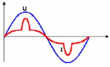
The rate of current harmonic distortion is an electrical parameter which defines the overall distortion of the magnitude of the sine wave and the level of pollution from a power grid.
