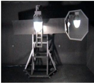
The basic measurement done in lighting product photometric test is the luminous intensity at specific planes and angles. Two different
